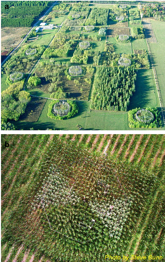
Fig. 1. The two Free Air CO 2 Enrichment (FACE) experiments on agroforestry tree crops: a) The AspenFACE experiment in Rhinelander, Wisconsin (USA) where elevated CO 2 and elevated O 3 treatments are tested alone or in combination (field station with 12 experimental plots, photo by Dave Karnosky) and b) the POP-EUROFACE experiment in Tuscania, Viterbo (Italy) where elevated CO 2 treatment and N fertilization treatments are tested alone or in combination (particular of one experimental plot, photo by Steve Bunn).
