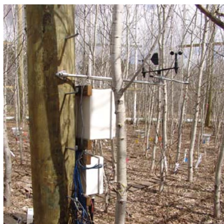
Control panels for the intensive micrometeorological monitoring in each Aspen FACE ring were repositioned on the new center poles.
