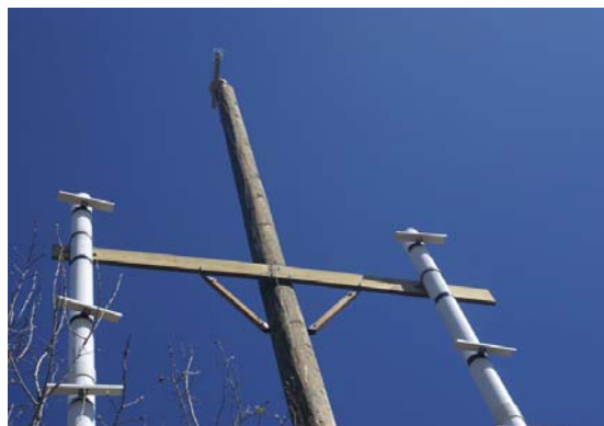
PAR sensors were replaced at the top of vertical vent-pipe-support poles.
