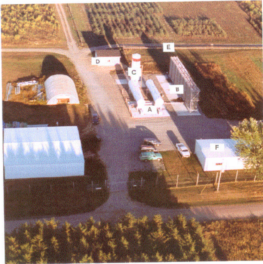
FIGURE A-2. Central Control Systems for CO 2 , Liquid O 2 , O 3 Production, and Gas Distribution (from Dickson et al. 2000) A. Liquid CO 2 storage tank. B. Ambient air heat exchangers. C. Liquid O 2 storage tank. D. O 3 generation building. E. CO 2 and O 3 gas distribution lines. F. Main computer control building and shops.
