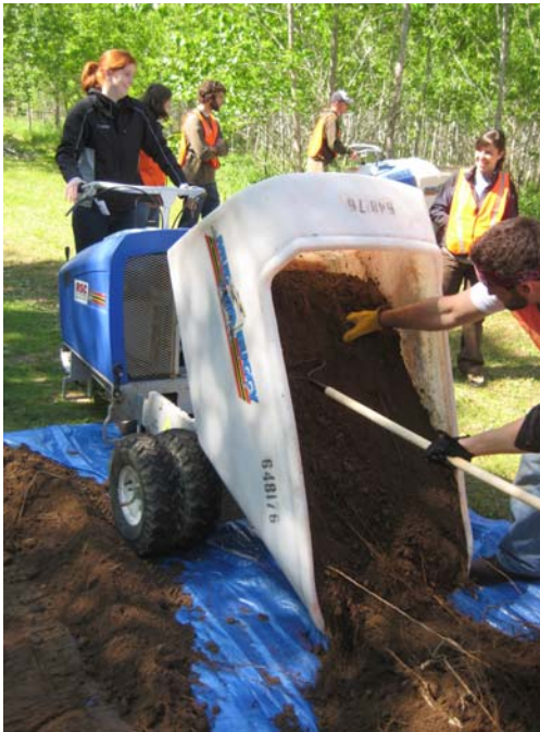
Commercial “mud buggies” were used to forward the soil from inside each ring to the large soil sieves used to separate coarse roots from soil.
