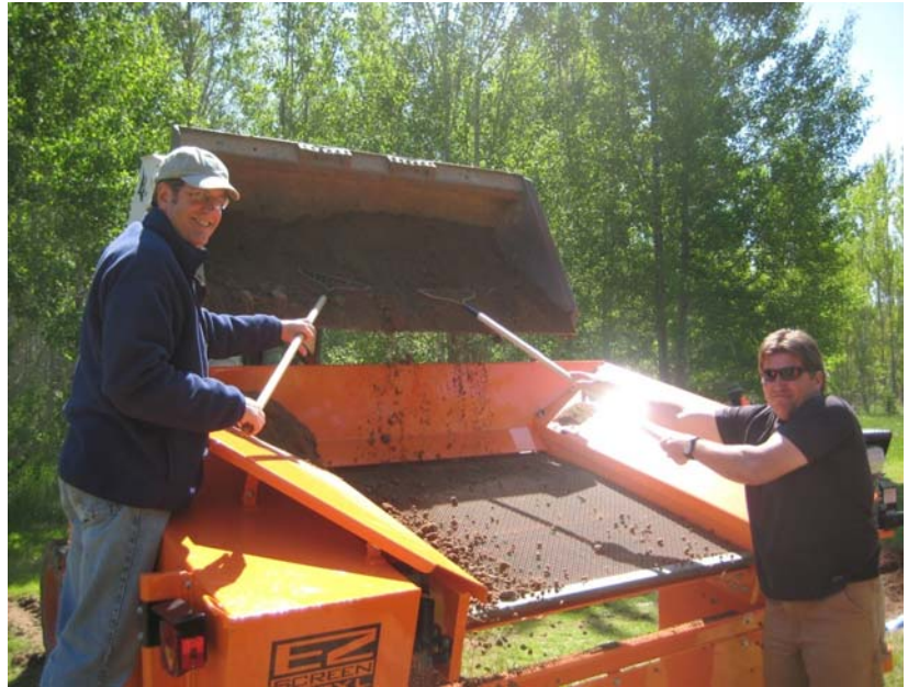
Long-time FACE Principal Investigators Kurt Pregitzer (University of Nevada) and Don Zak (University of Michigan) test the operation of the commercial soil sieve on June 9, 2009. The sieves worked very well and were used to separate coarse roots from soil.
